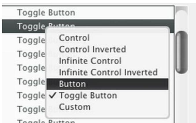
To configure a knob or slider, select 'Controls' from the popup, until the list columns change to 'Control'. Decks are listed as left(A) right(B) and C,D,E. Then when an item is selected, move a knob or slider to set it.
