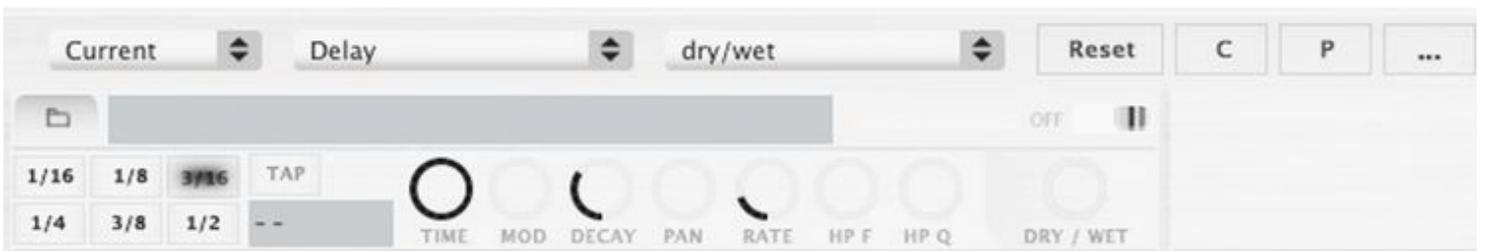
Then select a parameter from third popup of the editor, most common parameter is dry/wet which controls how audible the effect is (dry is unaffected, wet is fully effected).
