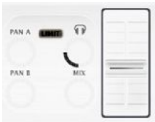
Pan knobs, headphone gain knob, headphone mix knob and master volume slider.
